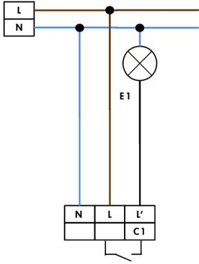
Standard mode with 1-channel motion detector with permanent light function
