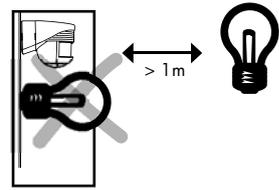
3) Minimum distance to switched lighting, frontally or laterally to device: 1 m
