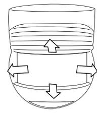
By swinging the sensor head horizontally (ca. 90°) and vertically (ca. 85°) detection area can be changed.
