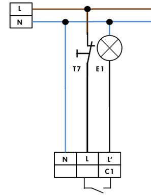
Parallel connection with 1-channel motion detectors
