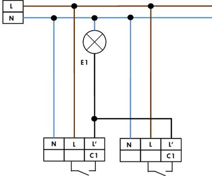
Standard mode with 1-channel motion detector (e.g. stairs)
