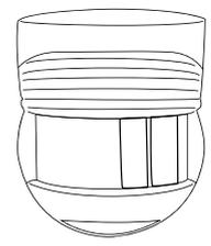
If necessary, the lens segment(s) corresponds to unwanted detection zones may be masked with the enclosed covers to reduce the field of vision.
